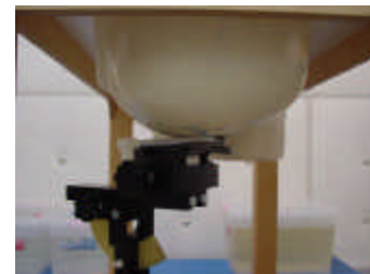
Fig. 17. Head SAR Test Setup
