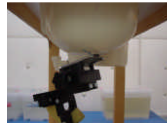
Fig. 18. Head SAR Test Setup
