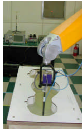
Figure 4. Photograph of the probe and the Phantom
