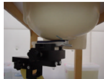
Fig. 17. Head SAR Test Setup
