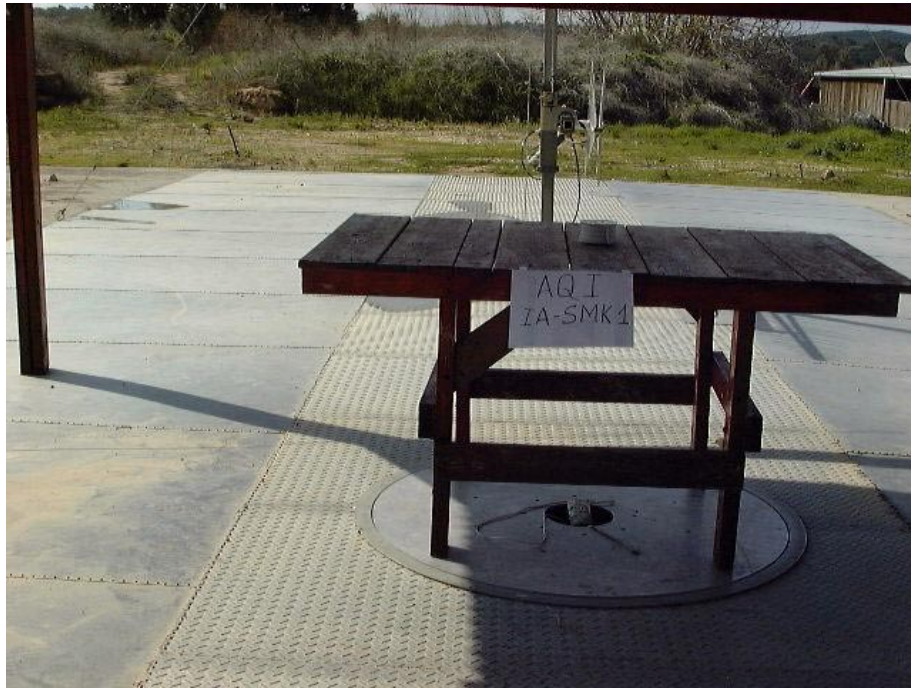
Figure 1. Spurious Radiated Emission Test. Front
