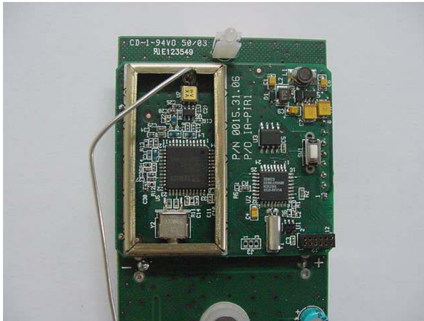
Figure 52 PCB Side 1 Area Under Shield
