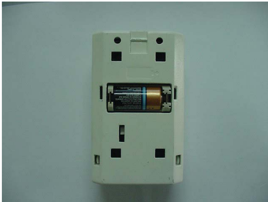
Figure 47 Rear View Battery Cover Removed
