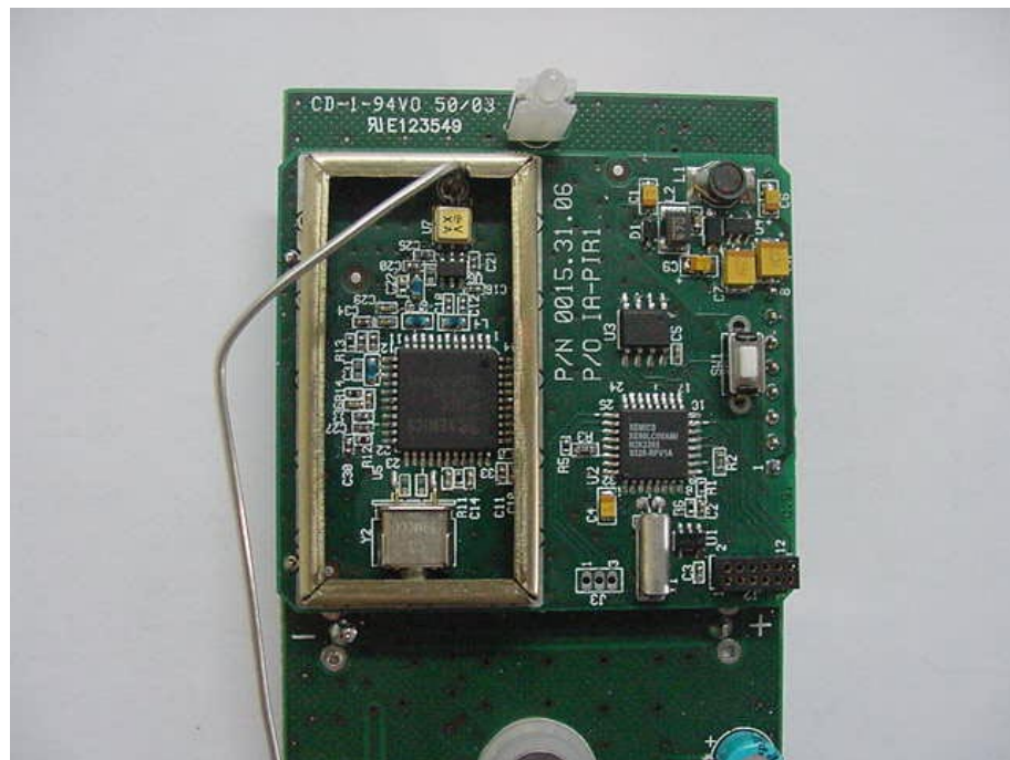
Figure 5 PCB Side 1 Area Under Shield
