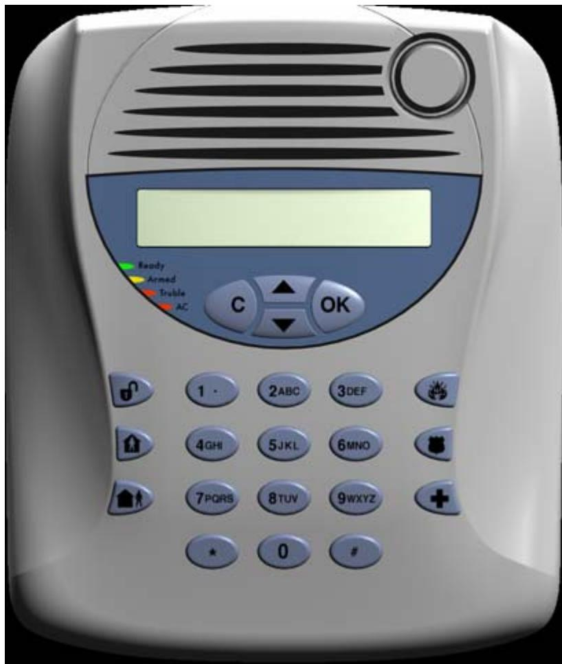
3.2.1 The Control Panel keypad is made of a single semi-transparent silicon rubber mask with back-light keys arranged in four groups as follows:
