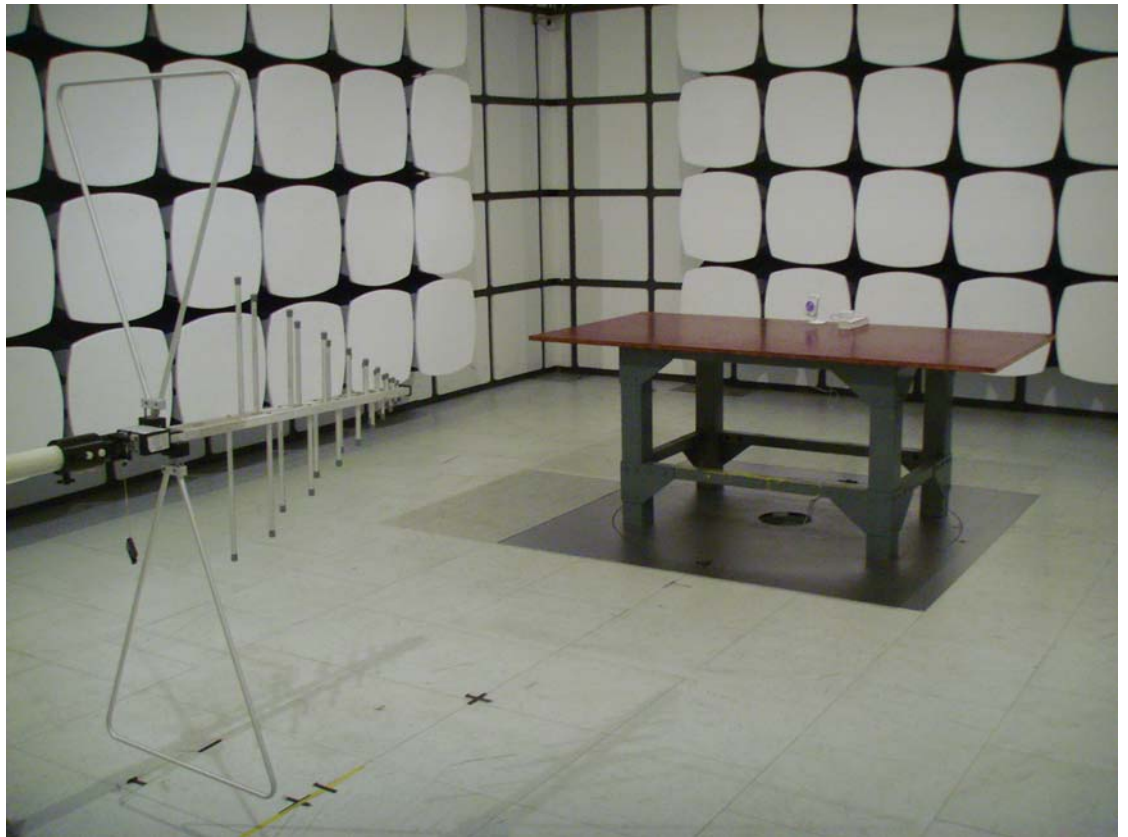
Radiated Emission Test Setup:
