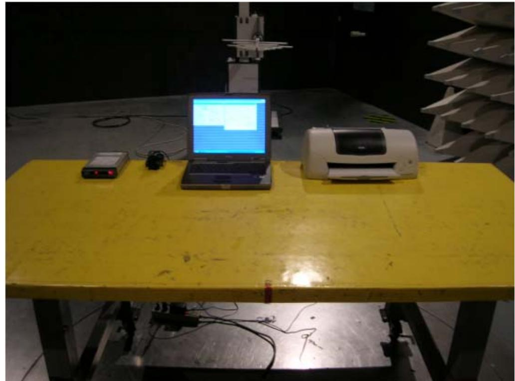
**Radiated Emissions (1GHz~10th harmonic of highest frequency)**
