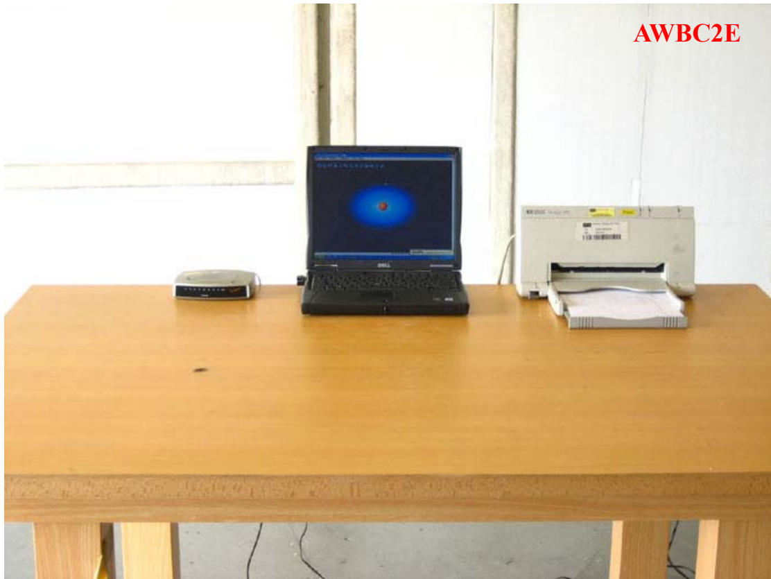
Photo 1: Radiated Emission Test set-up photo
