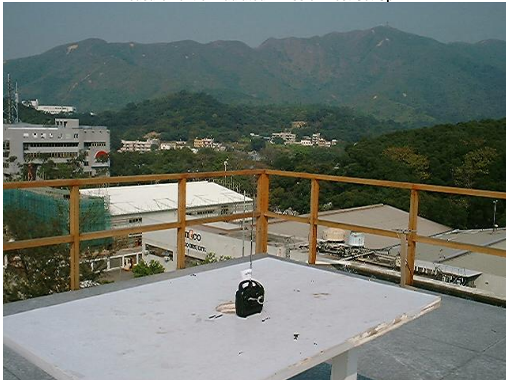
Measurement of Radiated Emission Test Set Up
