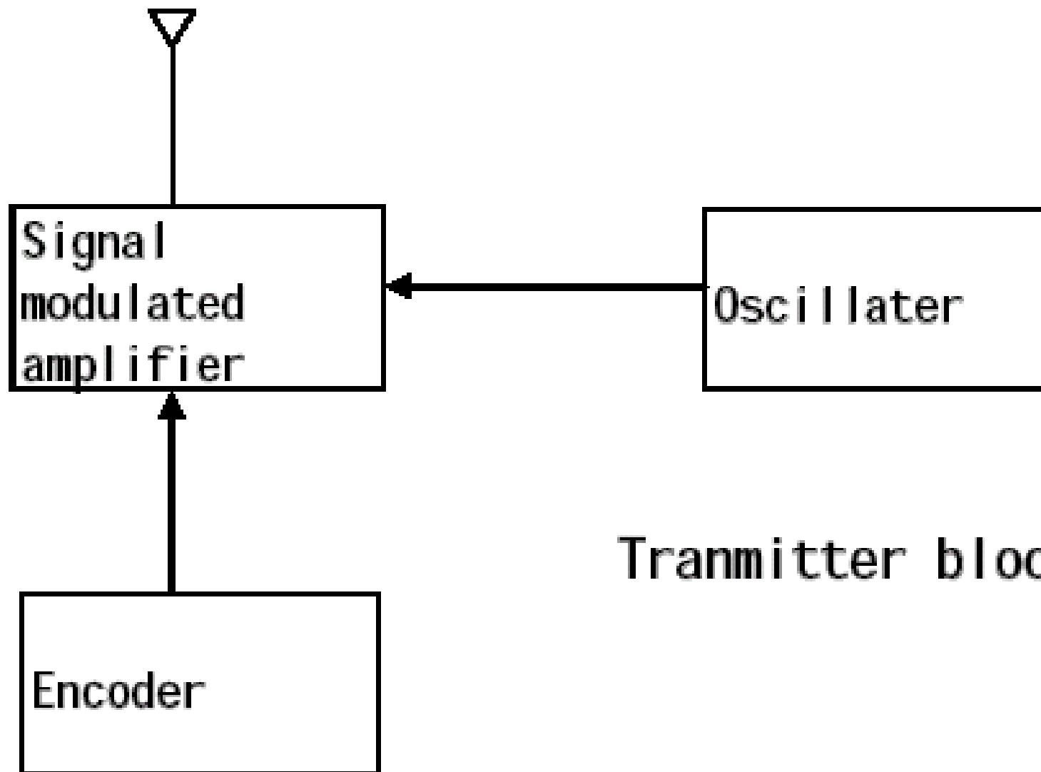
Transmitter block diagram
