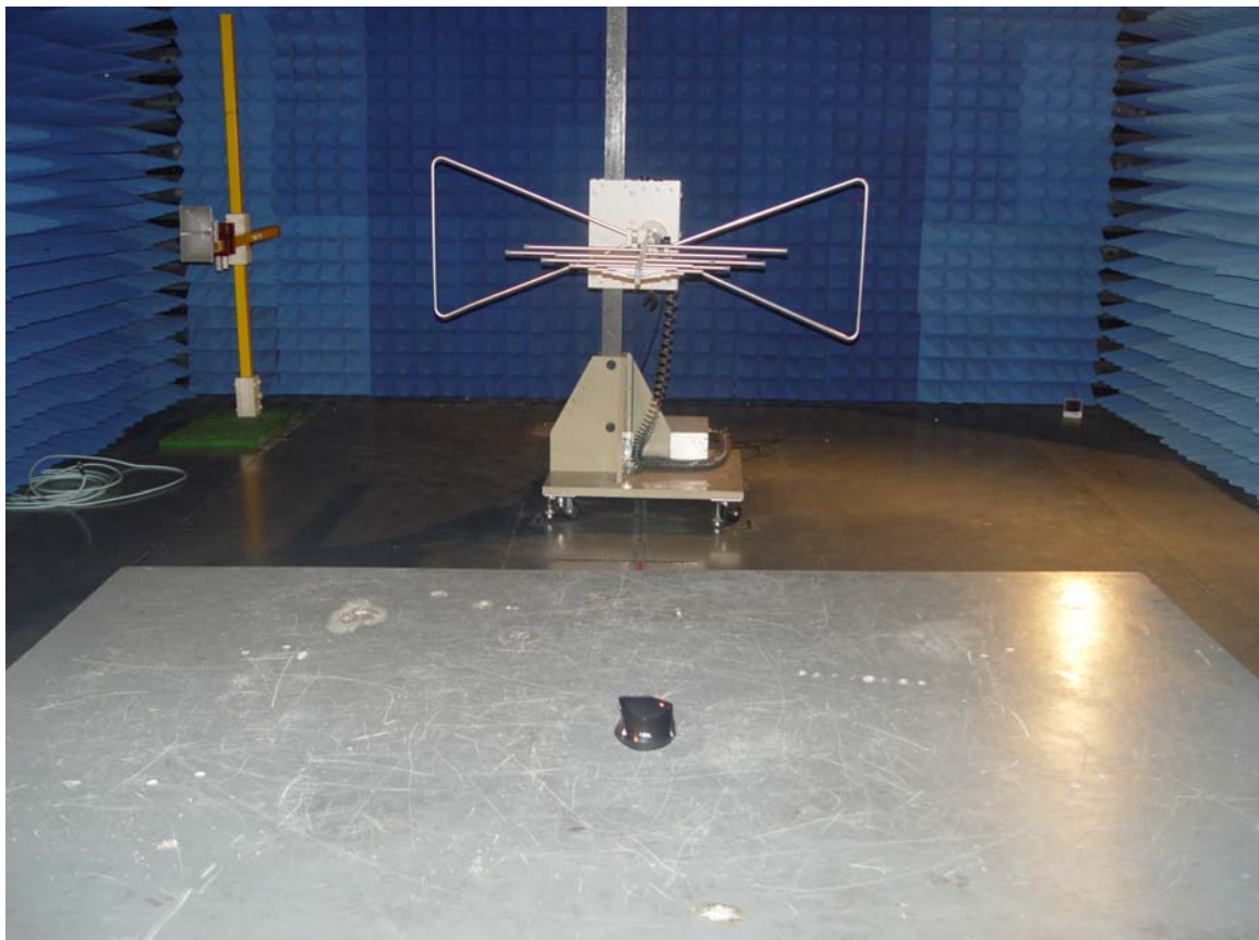
Radiated emissions test 30MHz- 1GHz
