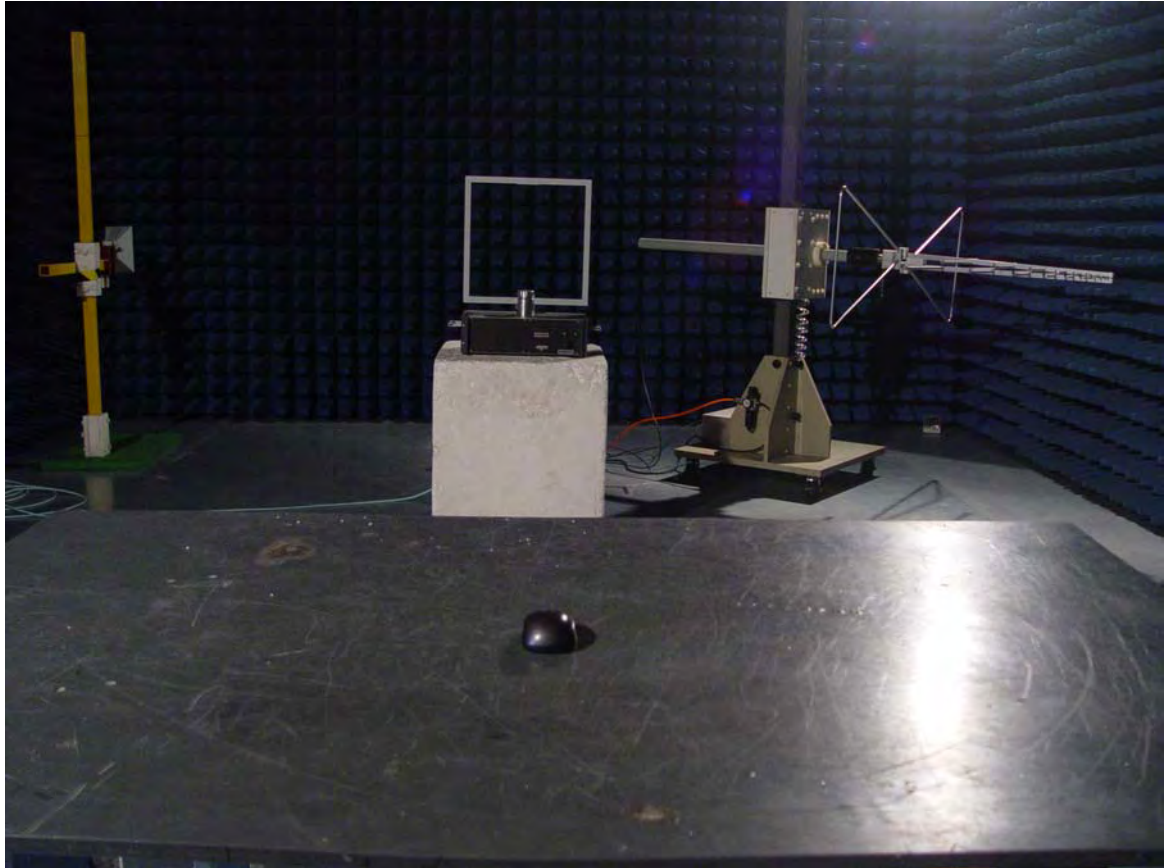
Radiated emissions test < 30MHz
