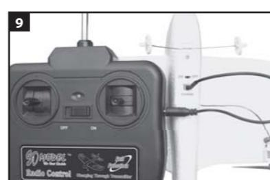
9. Make certain right and well connected, switch "ON" the "ON/OFF" switch on the transmitter. If it is charging, the signal light should be sparkling. After 13-15 minutes, the battery in the airplane is full charged, then the signal light keep bright. Switch "OFF" position, push out the wire. Notice: Must disconnect in time, forbid keeping charging when the battery is full at the first time charge. Plane will climb steadily.
