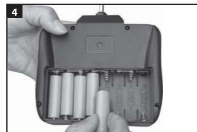
4. Insert eight "AA" alkaline batteries. Be careful of the electrode mark on the socket, don't put the batteries at the wrong electrode.
