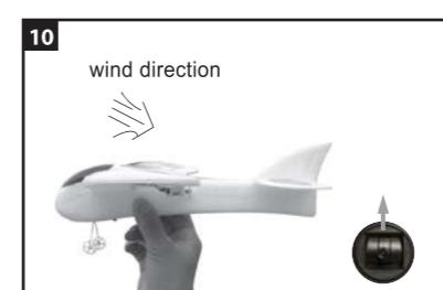
10. Hand launching: Model must be heading the direction of wind. After switching on the power of radio, then turn on the power of airplane. Push the throttle control up of the transmitter to make the propeller running in full speed, then throw the plane at straight direction toward the direction of wind. Plane will climb steadily.
