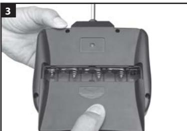
3. Remove the batteries cover on the bottom of the transmitter.
