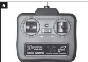
6. Switch "ON" the "ON/OFF" switch on the transmitter. If the LED light on the transmitter is shining, means the transmitter is working or not, you need check if the batteries is undercharged, and make sure you fit the batteries in the right way.
