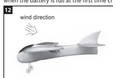
12. Choosing the plane to land at head wind position. Turn off or slow down the propeller speed, the model will decline steadily for landing.
