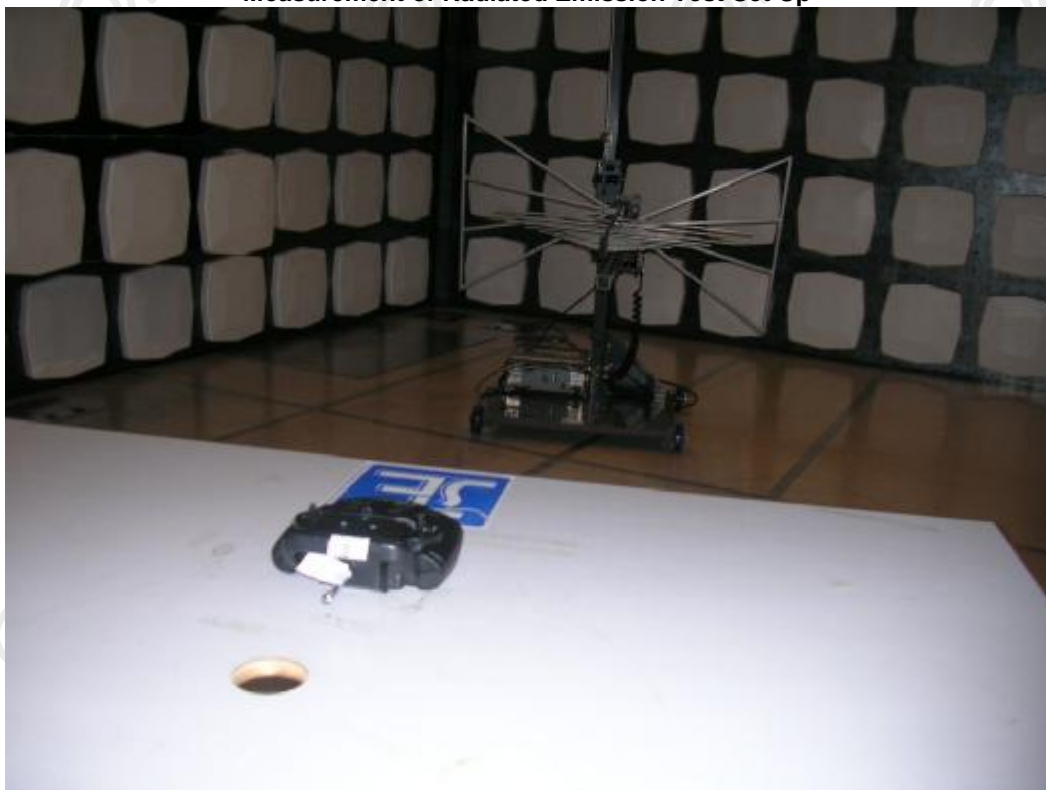
Measurement of Radiated Emission Test Set Up
