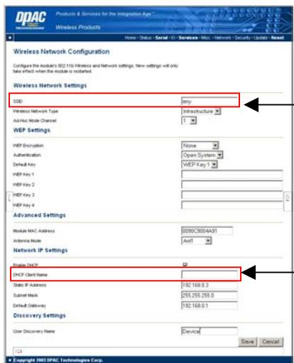
In the Module Web interface, click the **Network** link at the top of the page. The Wireless Network Configuration page appears.
