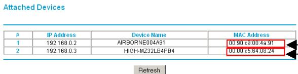
The row with the device name **Airborne** shows the Module's IP address, device name, and MAC address (the MAC address follows the word **Airborne** and appears on the back of the Module enclosure). Record this IP address below, as you will need to reference it later.
