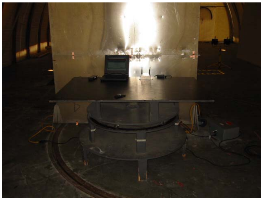
Power Supply Conducted Spurious Test Setup, Front View
