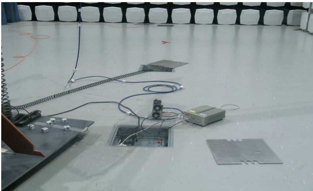
Band pass filter at the input of the amplifier is used in order to eliminate overloading the amplifier from the radiated power for 2 nd , 3 rd & 4 th Harmonics
