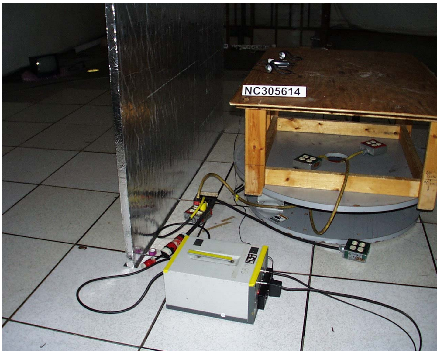
Test-setup photo(s): Conducted emission 150 kHz - 30 MHz
