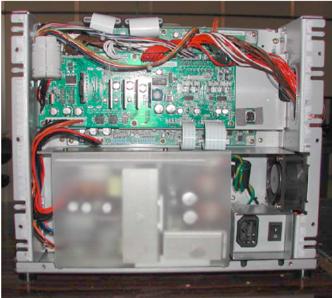
Photograph 13 - Internal Back View of the CV01-H01
