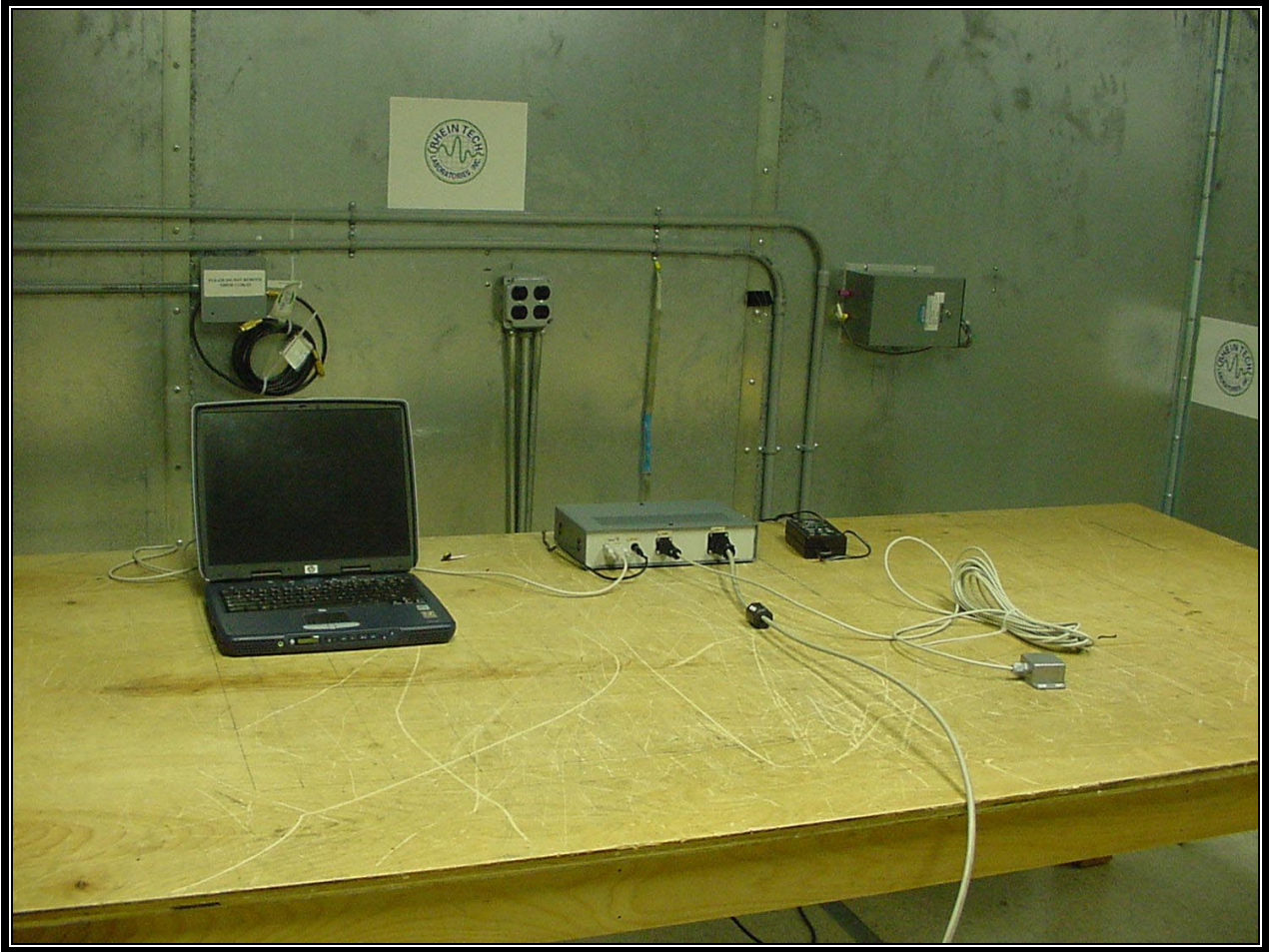
PHOTOGRAPH 7: CONDUCTED EMISSIONS FRONT VIEW DPU
