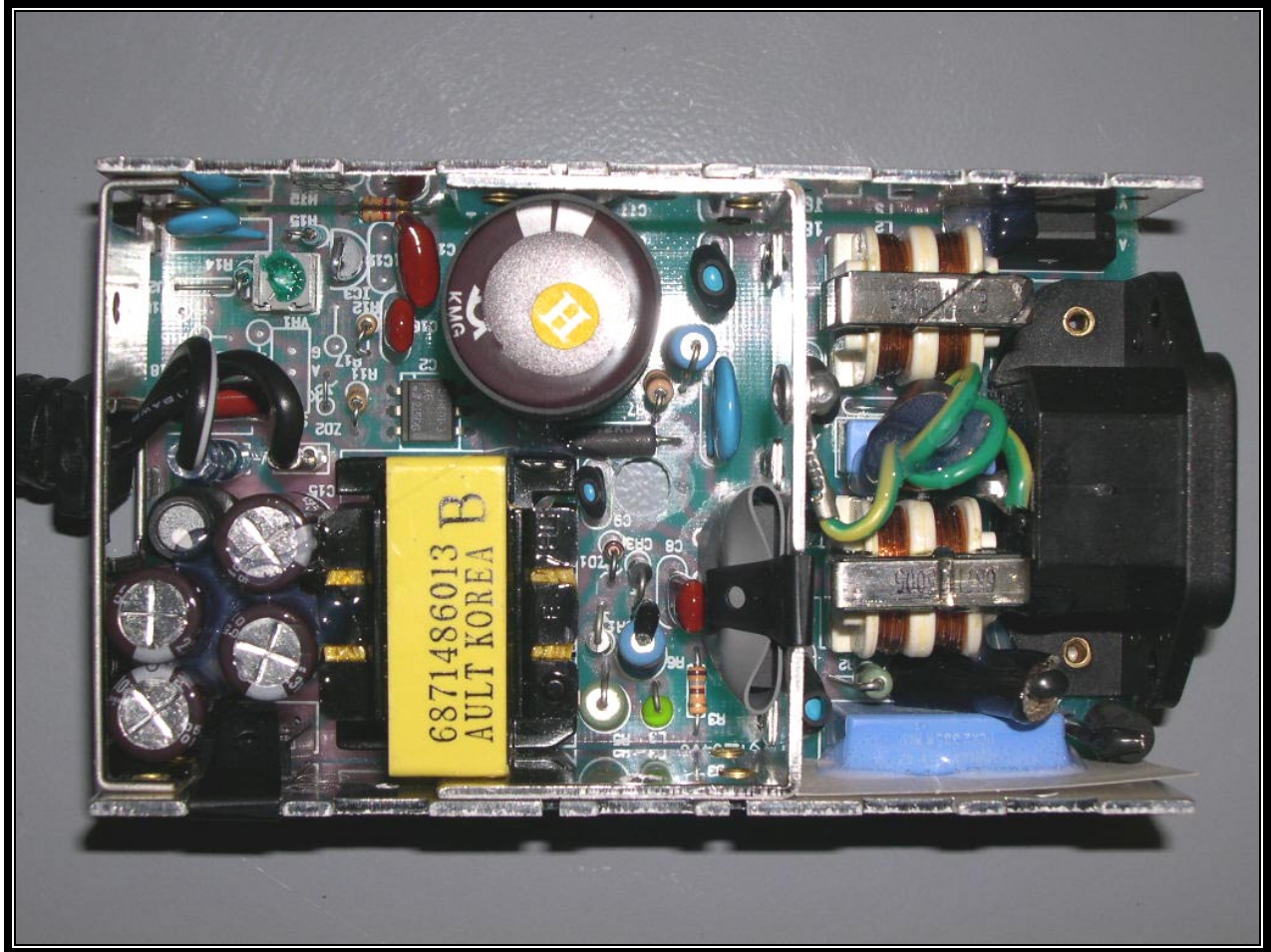
PHOTOGRAPH 42: POWER SUPPLY–TOP VIEW AC/DC CONVERTER
