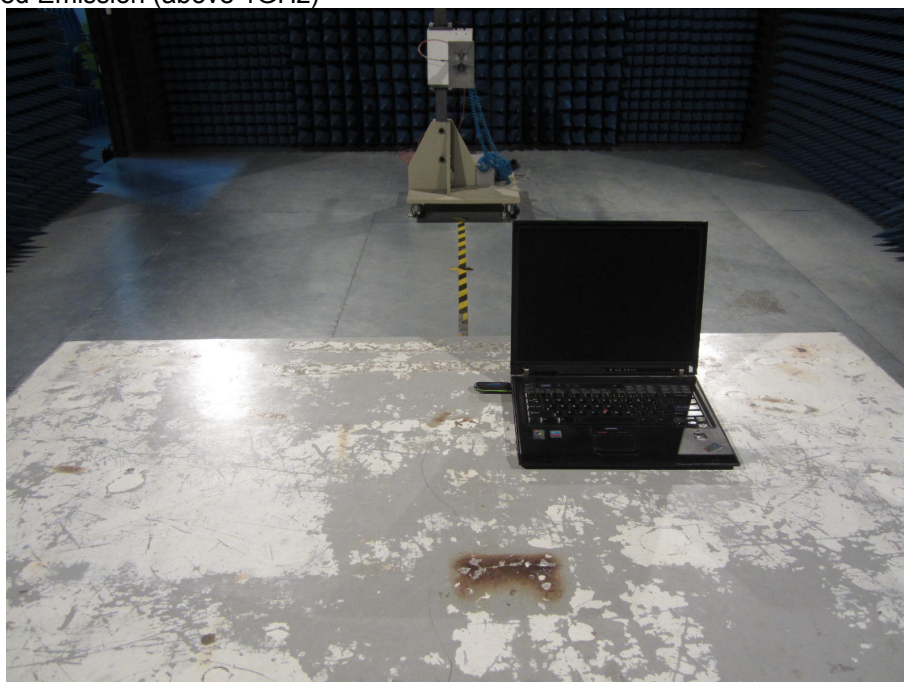
Radiated Emission (above 1GHz)
