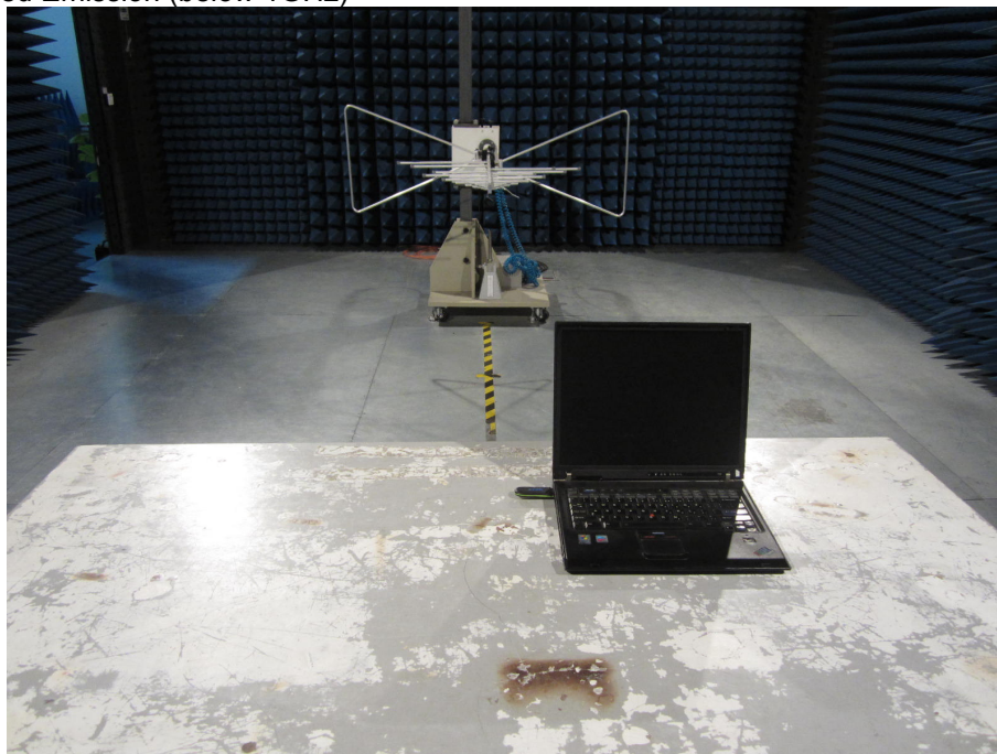
Radiated Emission (above 1GHz)
