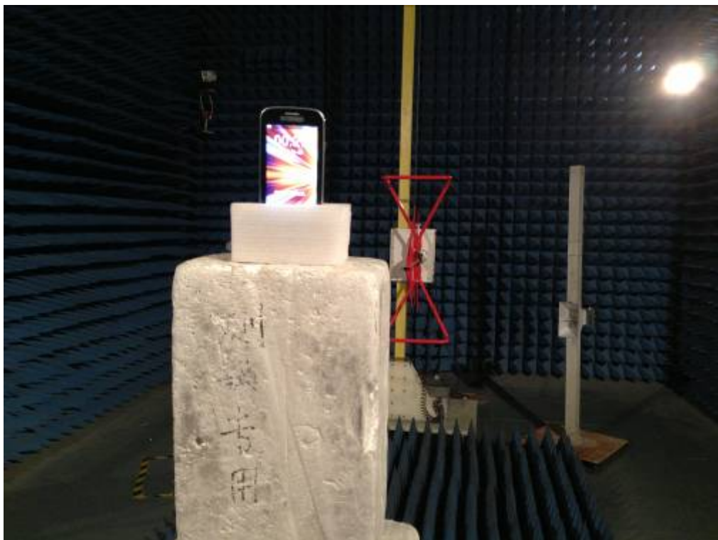
RADIATED EMISSION TEST SETUP
