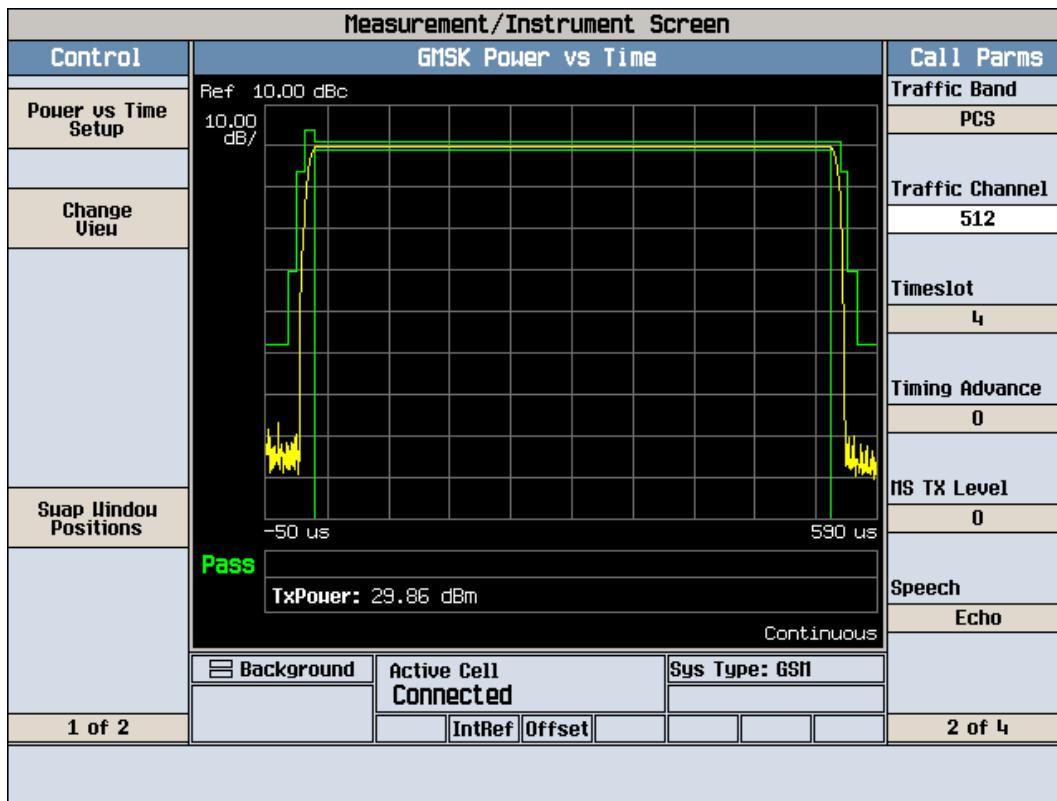
Power output conducted (GSM1900 661 CH)
