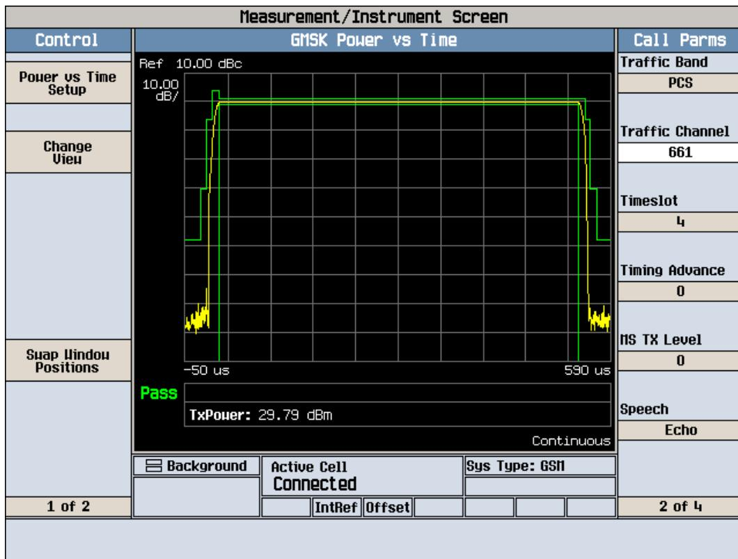
Power output conducted (GSM1900 810 CH)
