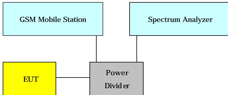
The level of the carrier and the various conducted spurious and harmonic frequencies is measured by means of a calibrated spectrum analyzer. The spectrum is scanned from the lowest frequency generated in the equipment up to 20 GHz.
