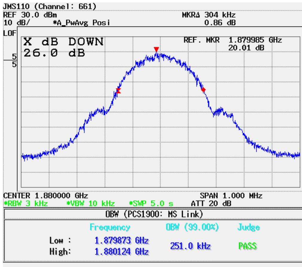
Occupied Bandwidth -26dBc BW (KHz) (GSM1900 810 CH)
