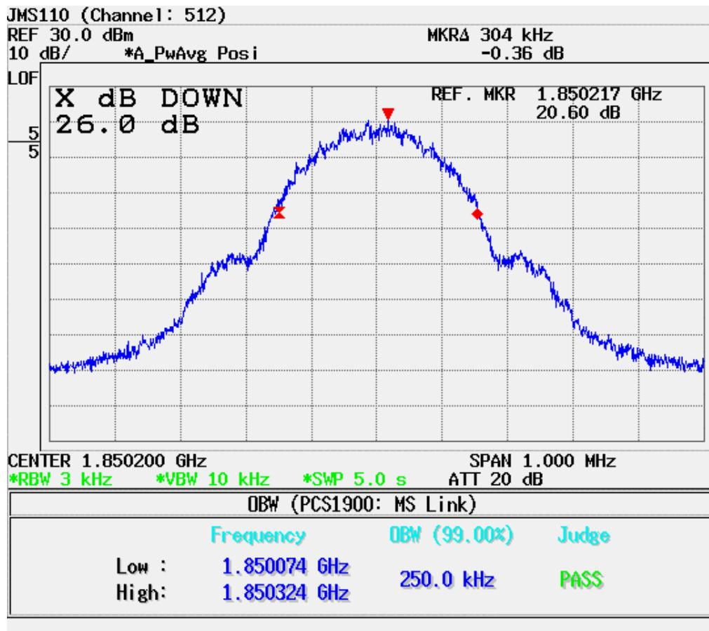
Occupied Bandwidth -26dBc BW (KHz) (GSM1900 661 CH)
