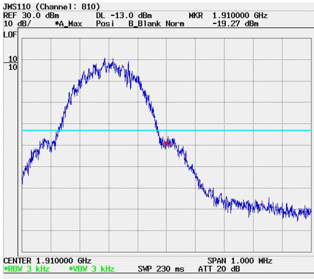
Power output conducted (GSM1900 512 CH)
