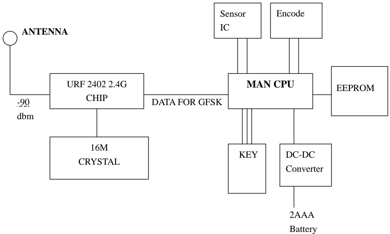
MCU will read the status of Optical Sensor, Encoder and Buttons, then control the RF chip by thru the SPI Bus, and the Modulation type of RF chip is GFSK, the frequency of Modulation is 150 KHZ, and the output power of RF chip is – 5dBm.
