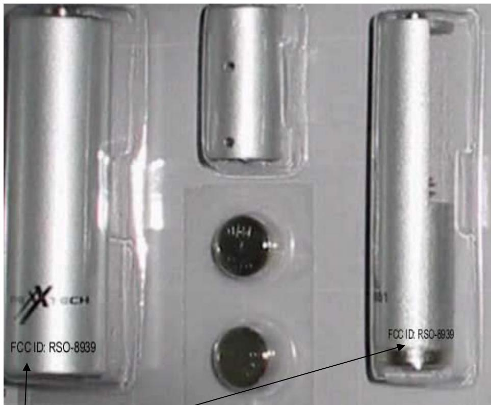
FCC ID printed on outside of device and FCC ID label printed inside battery compartment
