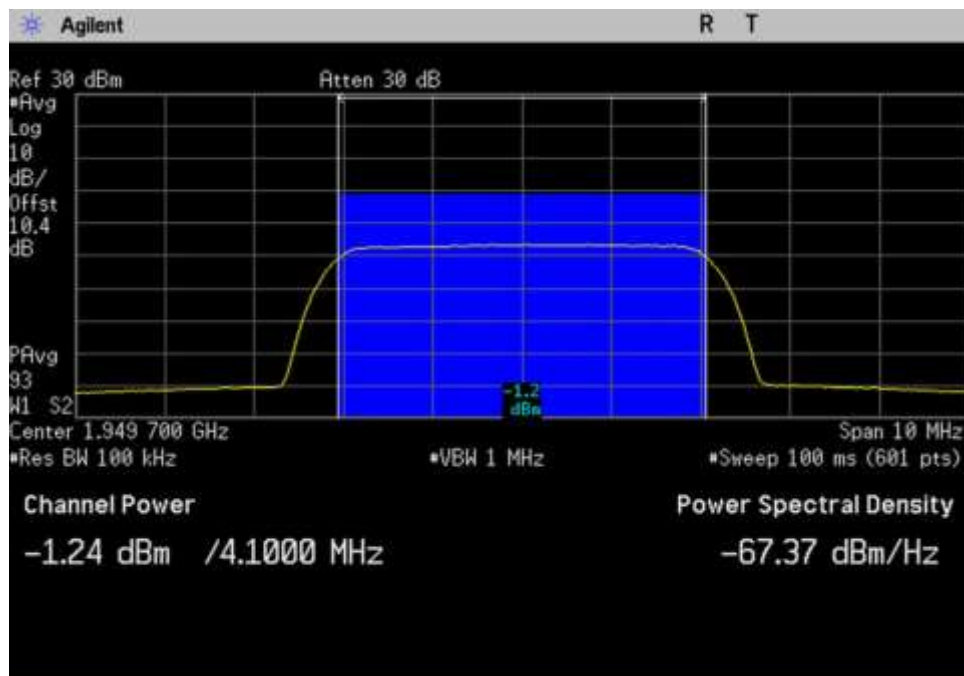
7.2-7.3 Power Gain_DL_1930-1995_AWGN_Max_ 1949.7MHz
