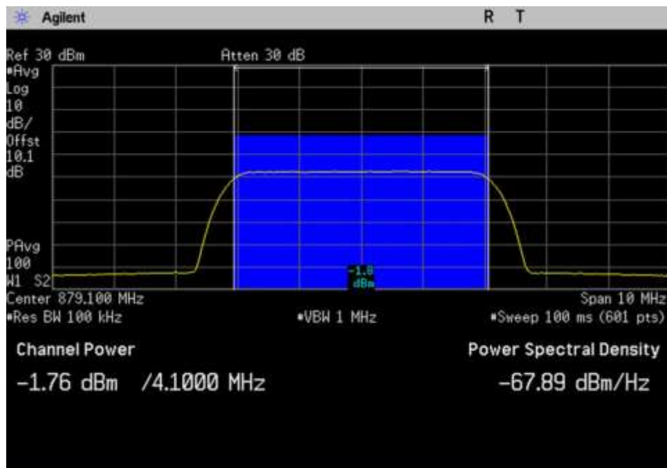
7.2-7.3 Power Gain_DL_869-894_AWGN_Max_ 879.1MHz
