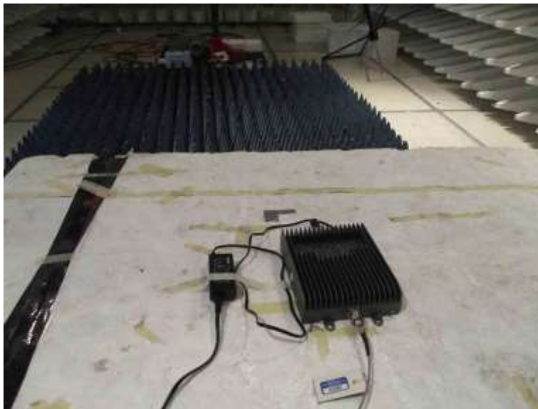
Section 7.12 Above 1GHz Cone placement Test Setup
