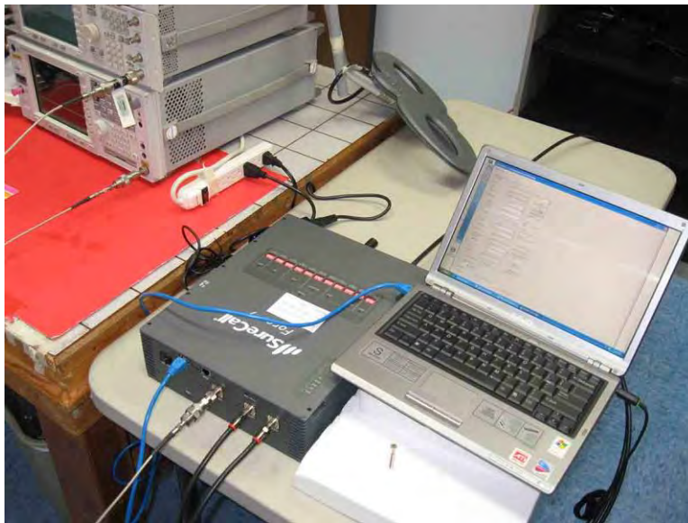
Section 7.8 Uplink Test Setup
