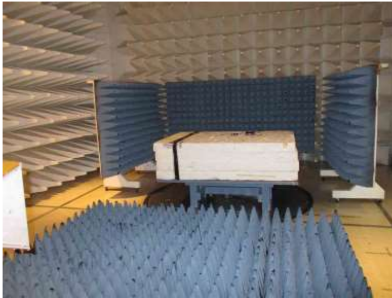
Section 7.12, Above 1GHz Cone placement Test Setup
