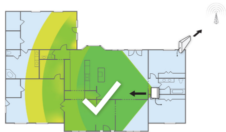
Face inside antenna away from outside antenna
