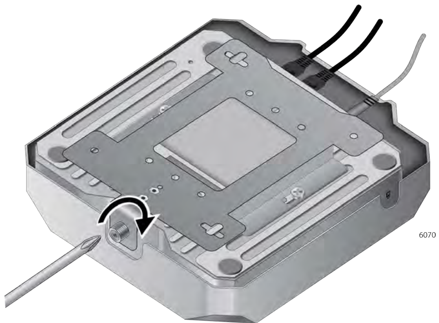
Figure 27. Tightening the Mounting Bracket Thumbscrew
