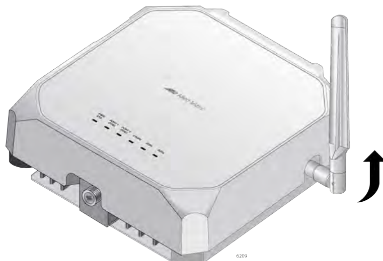
Figure 13. Adjusting the Antenna Position
