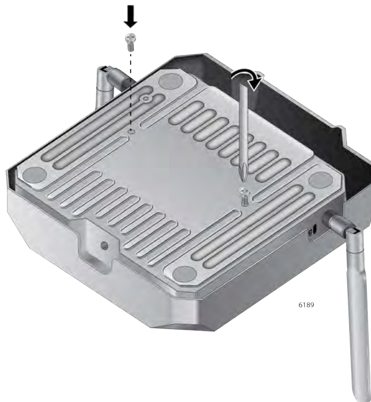
Figure 14. Attaching the Bracket Screws to the Access Point
