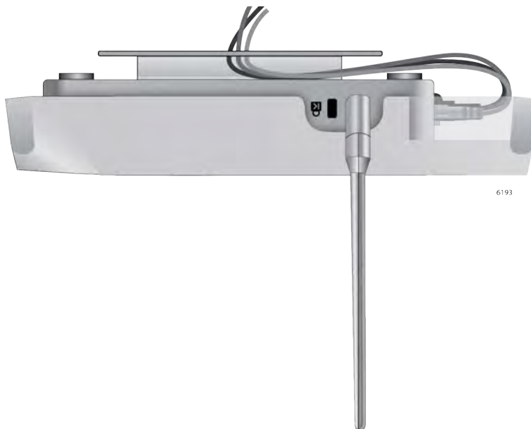
Figure 29. Fitting the Cables in the Cable Hide
