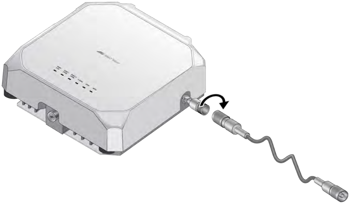
Figure 35. Attaching the cable to an Antenna Connector
