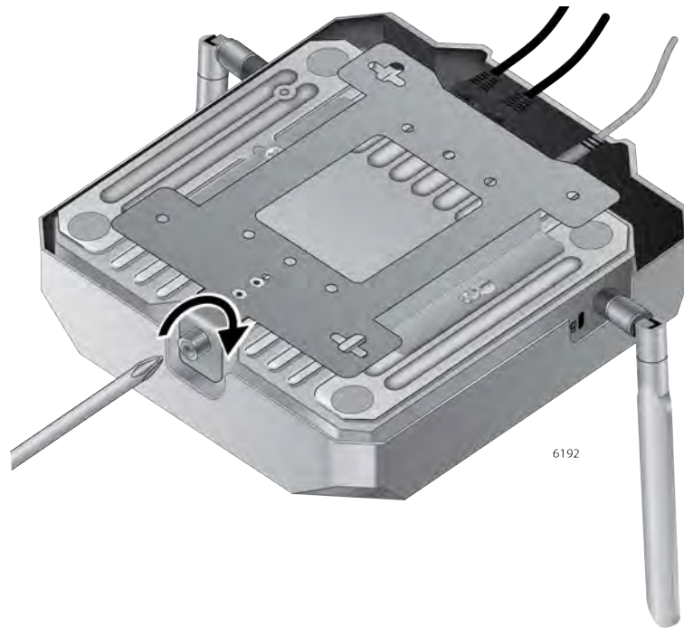
Figure 28. Tightening the Mounting Bracket Thumbscrew
