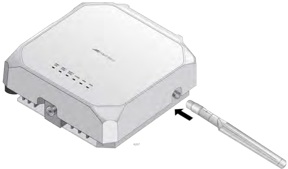
Figure 11. Aligning the Antenna to the Access Point
