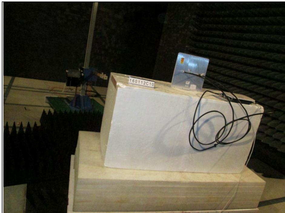
Radiated Emissions above 1 GHz Test (Test Mode B)
