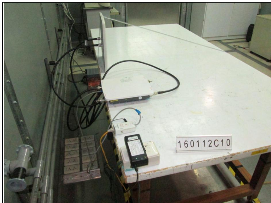
Conducted Emission Test (Test Mode B)
