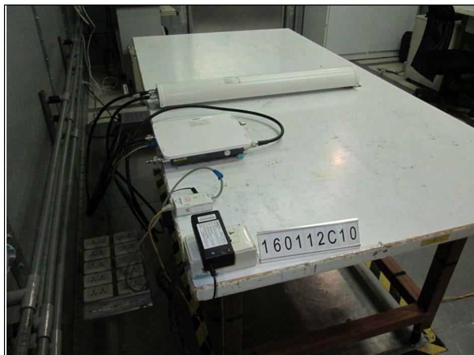
Conducted Emission Test (Test Mode C)
