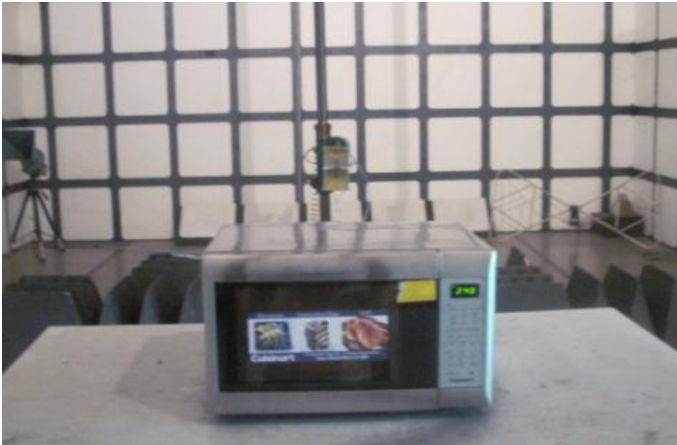
Operating Frequency Test Set-up
