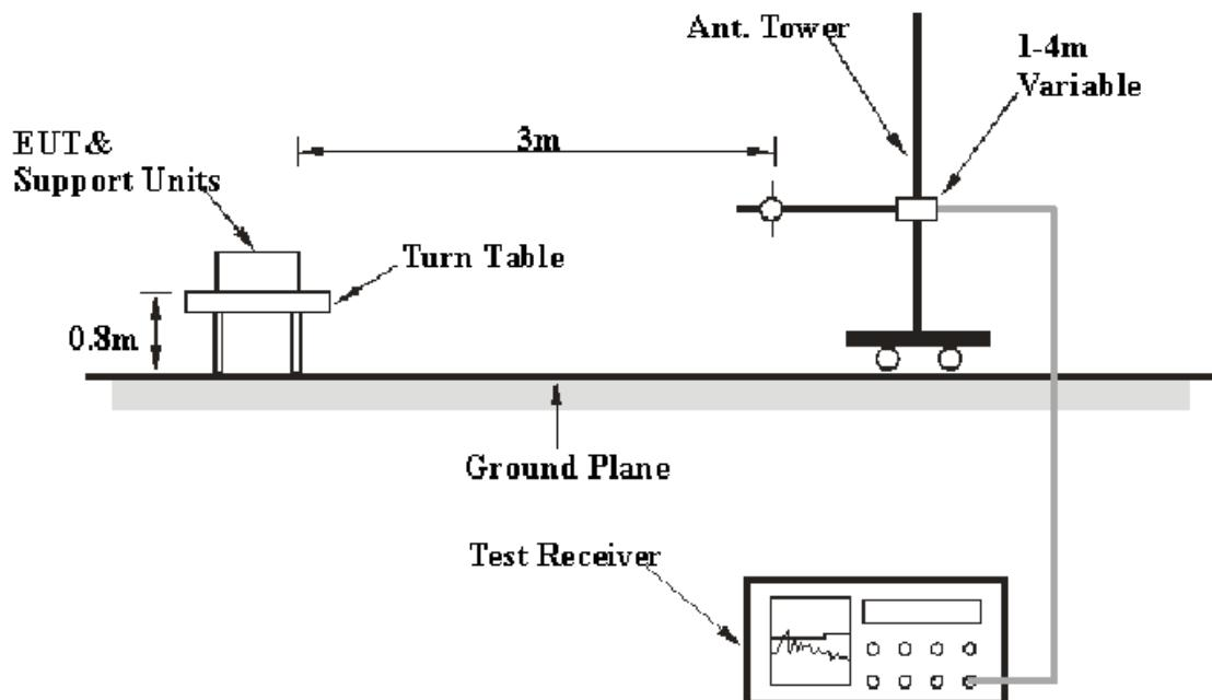
The radiated emission tests were performed in the 3 meters chamber B test site, using the setup accordance with the FCC MP - 5. The specification used was the FCC part 18.
