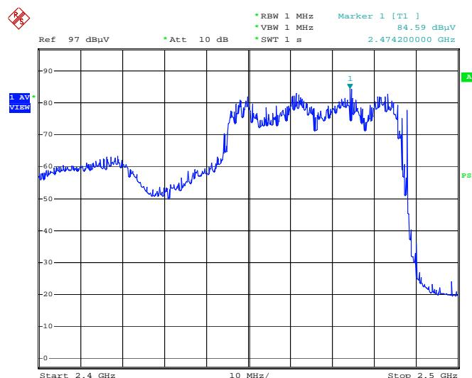
MD Microwave Oven 2M253J EM031A0W Frequency VS Voltage End
