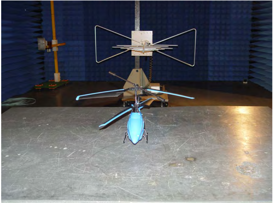
Radiated emissions test 30MHz - 1GHz
