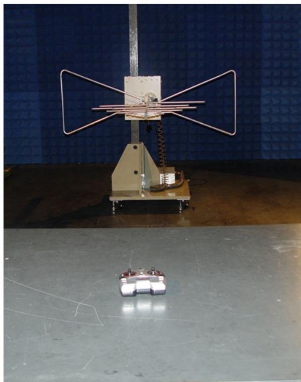
**Radiated emissions test > 1GHz**
