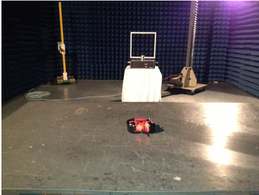
Radiated emissions test 30MHz- 1GHz
