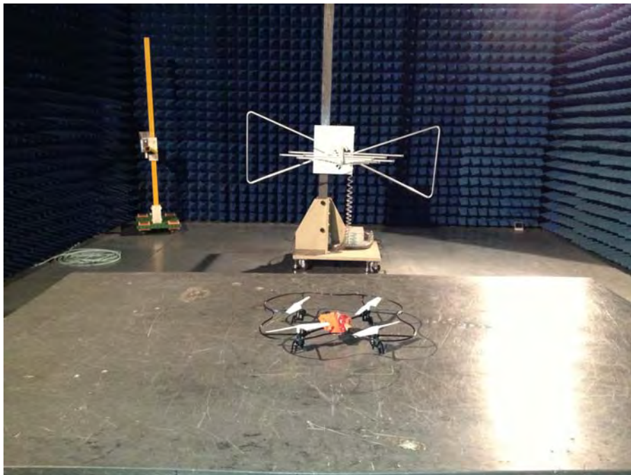
Radiated emissions test 30MHz- 1GHz
