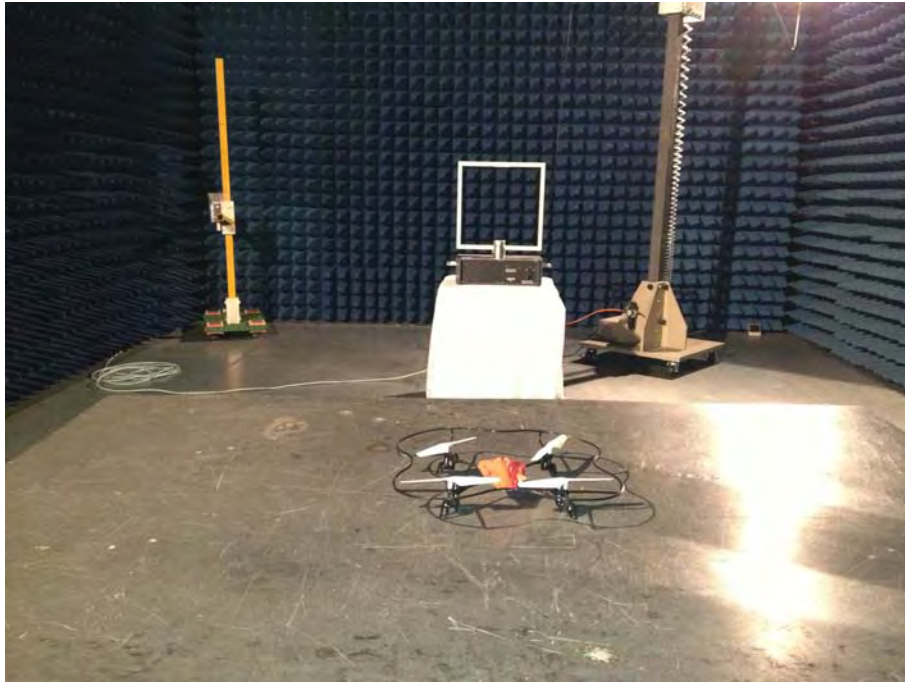
Radiated emissions test 30MHz- 1GHz
