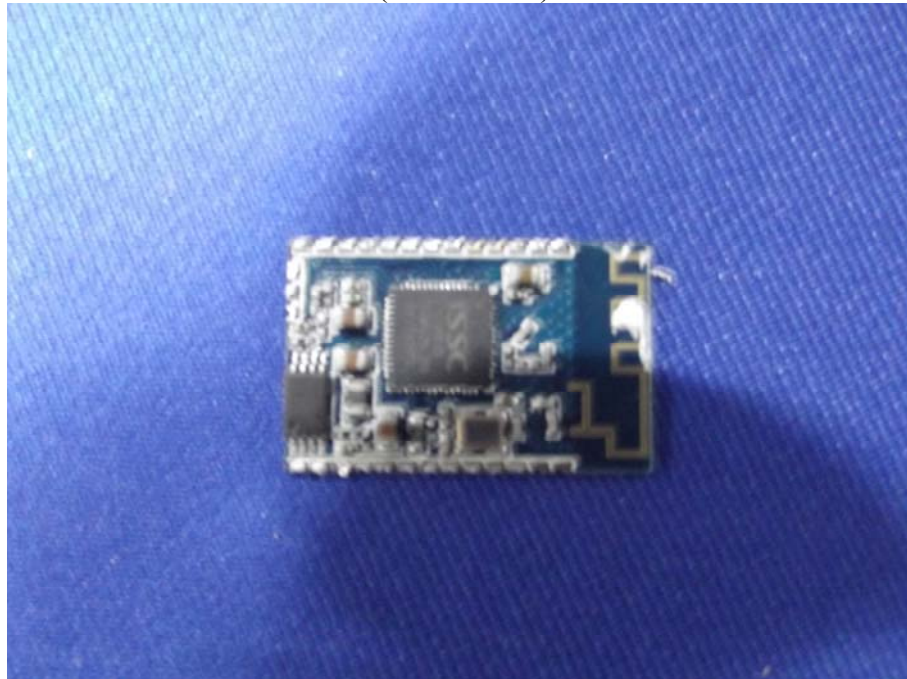
Figure 7 PCB of the EUT-Front View( BT module)
