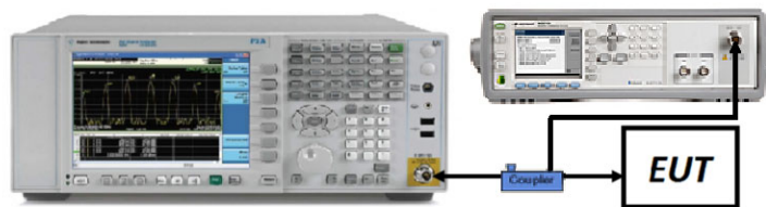
Figure 7-4. Test Instrument & Measurement Setup
