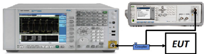
Figure 7-1. Test Instrument & Measurement Setup
