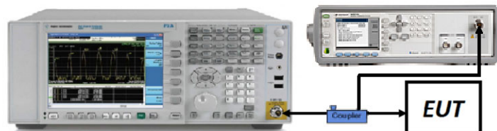
Figure 7-3. Test Instrument & Measurement Setup
