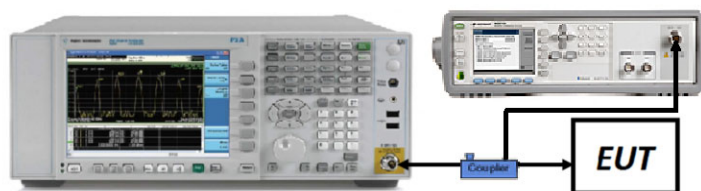
Figure 7-6. Test Instrument & Measurement Setup
