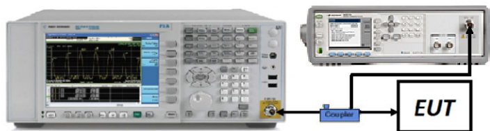
Figure 7-2. Test Instrument & Measurement Setup
