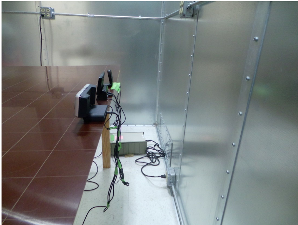
Test Configuration 1: Conducted Emissions, Endeavor with Home Cradle (side)
