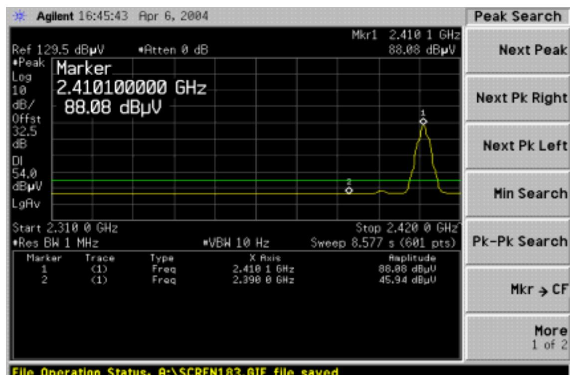
**Band Edges (DHT200 / CH High)****Peak measurement-Vertical**
