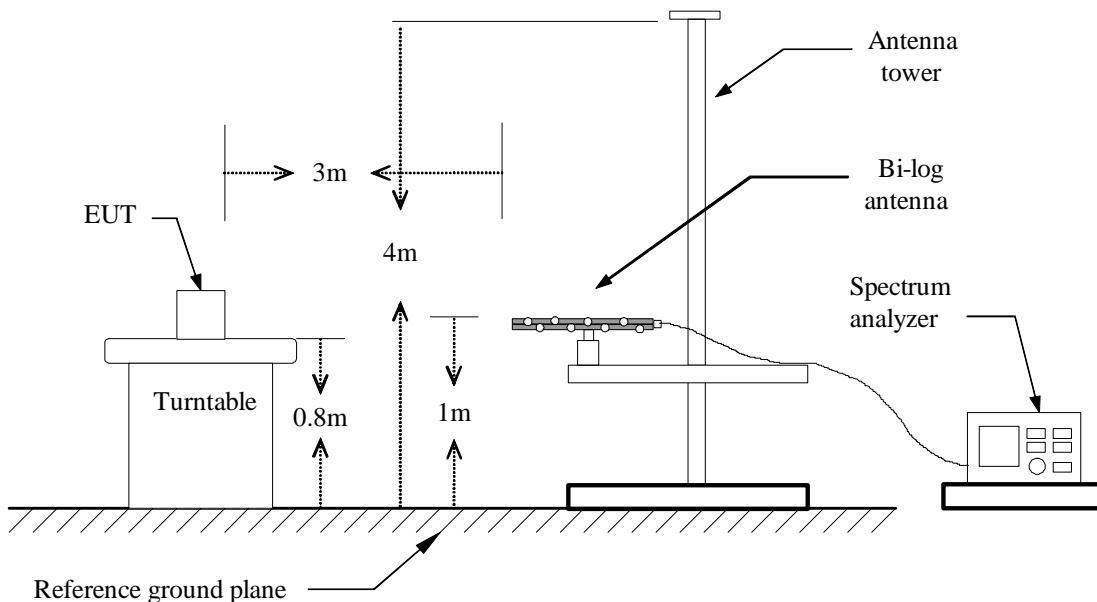
**Above 1 GHz**
