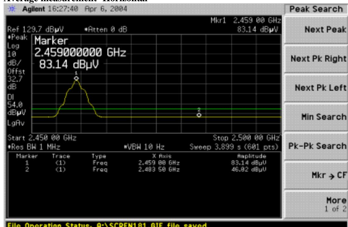
**Band Edges (DHT200 / CH Low)****Peak measurement-Vertical**
