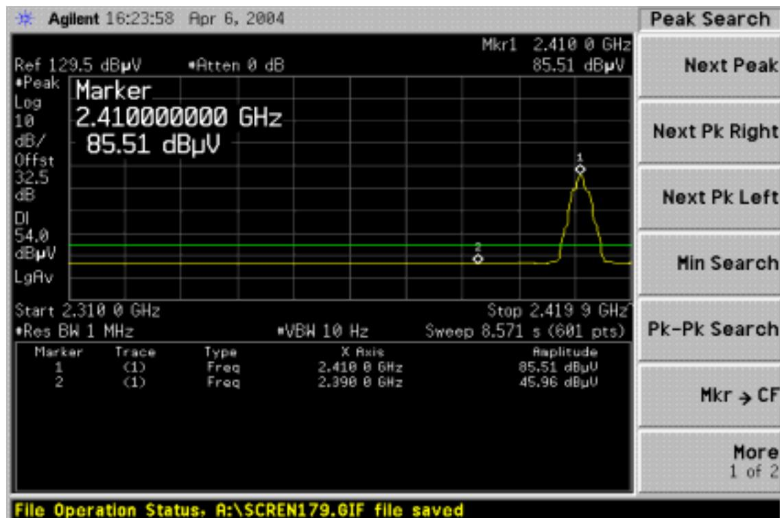
**Band Edges (DHT100 / CH High)****Peak measurement-Vertical**
