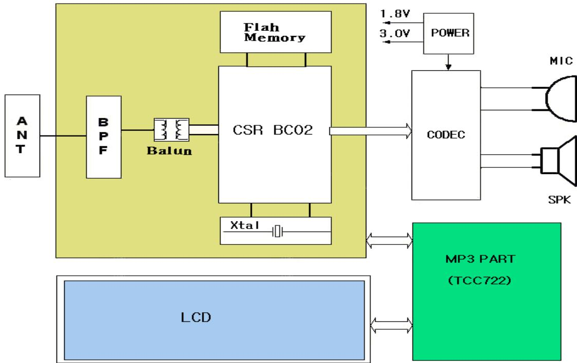
The Bluetooth functions of XBM-100P are controlled by TCC722 chip (MP3 core chip).
