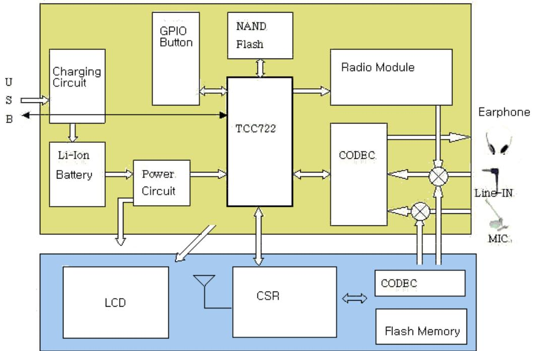
Lithium-polymer battery is built-in for power source. To charge, USB cable is used to connect on USB port of PC or another adaptor. On power circuit, 1.8V, 2.5V and 3.5V are created.
