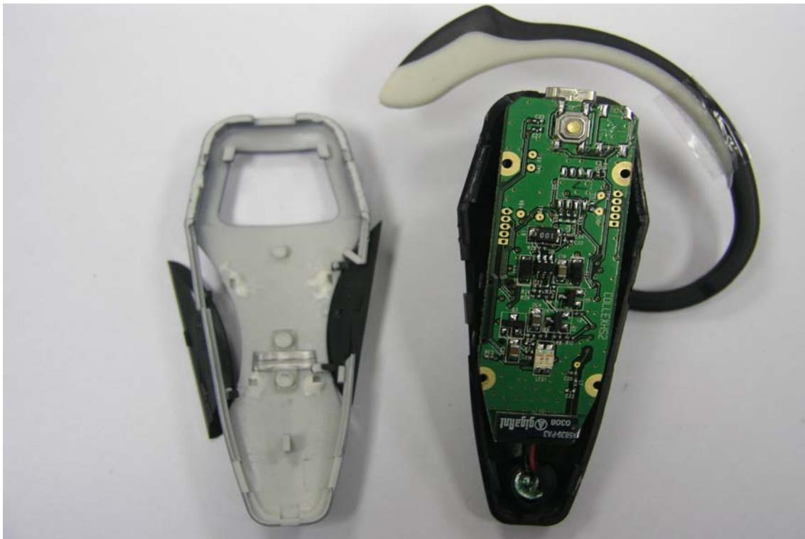
*Internal of EUT -1*
