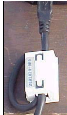
Fig. 9. Ferrite — Installed on USB Cable
