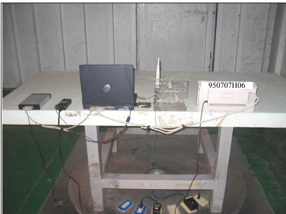
RADIATED EMISSION TEST (With Antenna 2)
