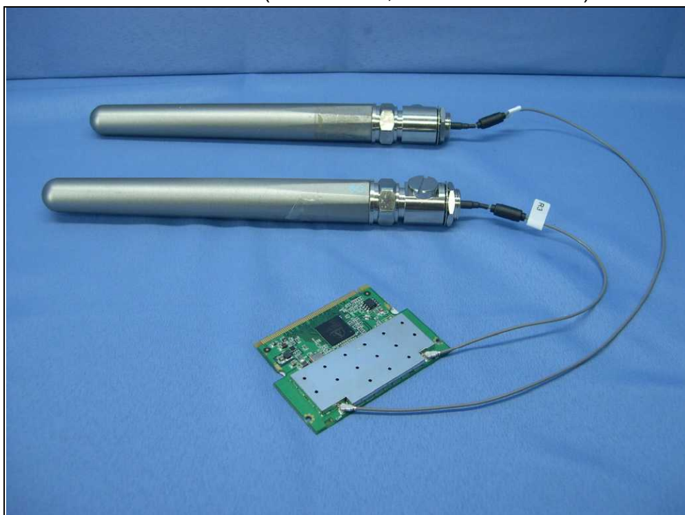
EUT + Antenna (without filter, Gain: 4.6dBi / 4dBi)
